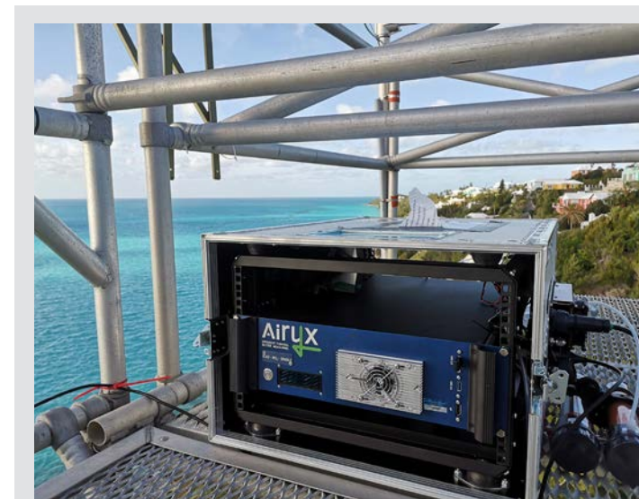
A high grade ICAD \text{NO}_x instrument purchased by the University of York. Customized with a special temperature stabilisation to adapt to the warm climate, the ICAD provides \text{NO}_x data for the BLEACH (Bermuda boundary Layer Experiment on Atmospheric Chemistry of Halogens) project.
