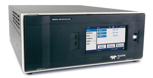
The Model 500 CAPS  $NO_x$  analyzer uses superior Cavity Attenuated Phase Shift (CAPS) Spectroscopy to measure True  $NO_{2'}$   $NO_{x'}$  and NO gases. The instrument combines direct  $NO_2$  measurements with highly efficient gas phase titration (GPT) to convert and measure the NO gas component. An automatic baseline reference cycle accounts and compensates for any potential baseline drift due to varying environmental conditions.
