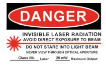
Instrument complies with 21 CFR 1040.10 and 1040.11
