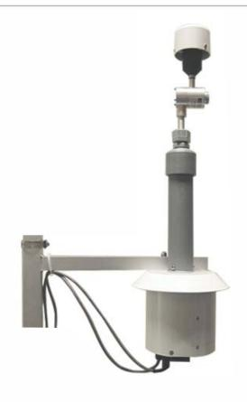
The NPM 3 is calibrated using 0.6µm NIST traceable polyspheres. These provide a critical and consistent baseline calibration. To correlate this calibration to real-world, non-spherical particulates, a Calibration Factor (K-Factor) is established by means of comparison to a collocated, trusted, and proven reference source (i.e., a BAM 1020) to ensure both accuracy and correlation.
