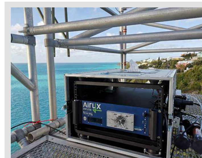
A high grade ICAD NO x instrument purchased by the University of York. Customized with a special temperature stabilisation to adapt to the warm climate, the ICAD provides NO x data for the BLEACH (Bermuda boundary Layer Experiment on Atmospheric Chemistry of Halogens) project.
