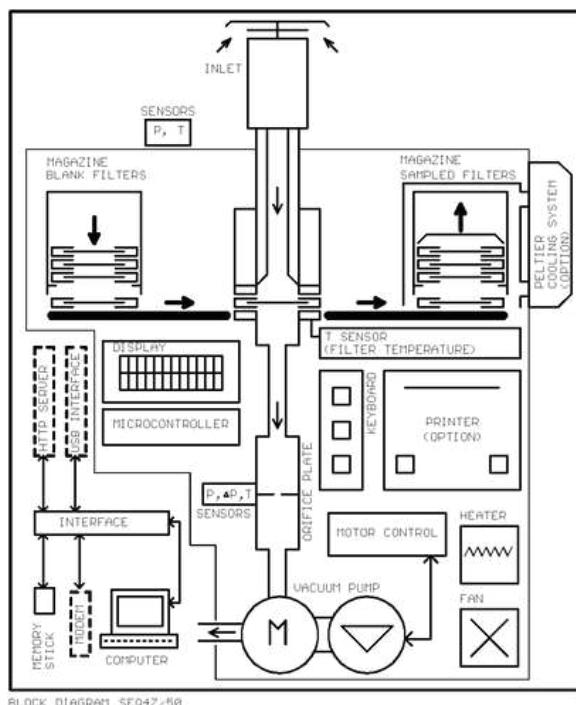
The **flow rate** of the SEQ47/50 is controlled in compliance with basic physical principles by means of a temperature- and pressure-compensated orifice plate according to Bernoulli's law and by conversion into operating- $\text{m}^3/\text{h}$  according to Boyle-Mariotte's law.
