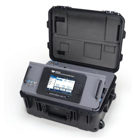
A portable, microprocessor based calibrator for precision gas analyzers, the Model T750 combines highly accurate mass flow controllers and compressed sources of standard gases to provide multipoint span and zero calibrations. UV ozone generator, photometer, and gas phase titration (GPT) chamber options are also available for the T750 for stable and accurate O<sub>3</sub> and NO<sub>2</sub> production.
