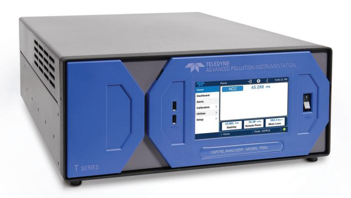
The Model T500U NO<sub>2</sub> analyzer is a significant advancement in the direct measurement of NO<sub>2</sub> using a Cavity Attenuated Phase Shift (CAPS) spectroscopy technique to provide highly accurate, real-time, continuous, and direct readings. The T500U offers a cost effective and low maintenance instrument package ideal for ambient and roadside monitoring.
