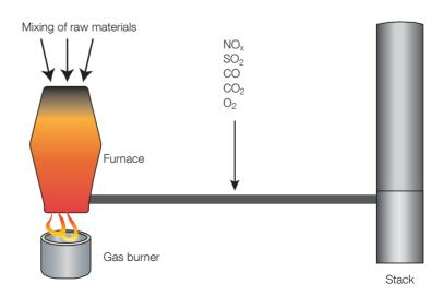
The measurement is made by a cross-stack optical sensor. The system can operate in high dust load and high temperature.
