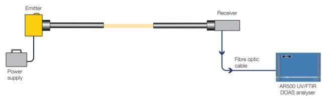
The OPSIS long-path air quality monitoring system brings new standards of accuracy and data quality to environmental monitoring. Every minute, several thousand cubic metres of air interact with the light between the light source - the emitter - and the receiver. When captured by the receiver, this light contains information on gases in the air it has penetrated.
