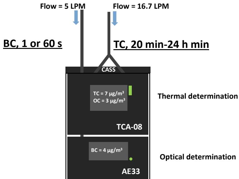
The TC and BC data are combined to yield the OC result by simple subtraction.
