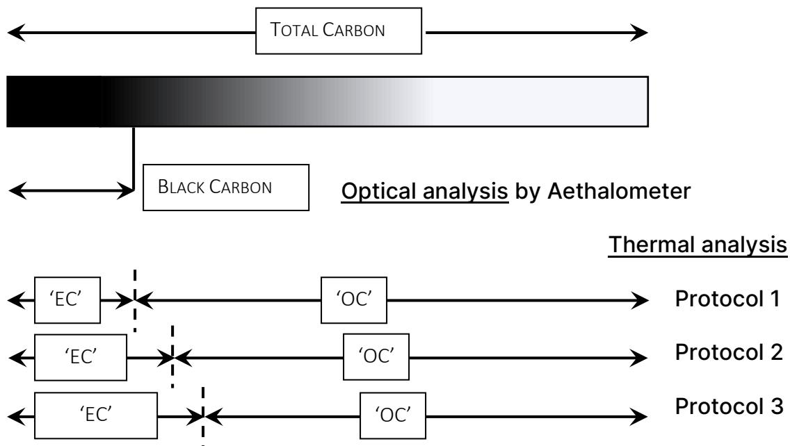
Thermal analysis methods usually agree quite well with each other for the determination of the Total Carbon content of the sample: but there may be substantial differences in the "EC/OC" partitioning, depending on the nature of the sample and the thermal protocol which is used for analysis.
