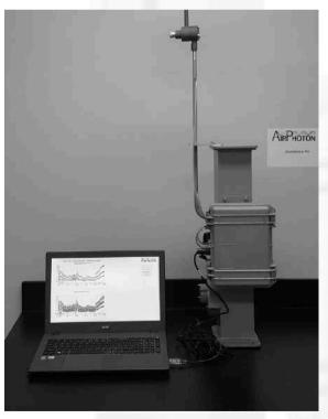
Our basic nephelometer designed for robust operation under a wide range of conditions. While its rugged design allows for field deployment, it is also a highly sensitive instrument which can be used in the laboratory or modified for use in aircraft. In this regard, the IN101T is highly versatile and can work in different environments and for different purposes.
