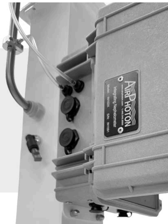
Dual pressure taps in inlet to provide accurate flow monitoring
