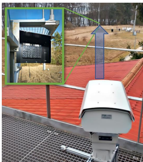
NH 3 Open Path Compact set up at the Federal Environmental Agency station Neuglobsow, Germany (left). Example data time series (right).
