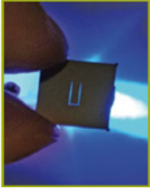
Ultra-sensitive patented optical cantilever microphone
