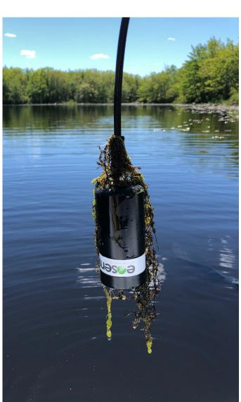
For researchers investigating carbon cycling in bodies of water, Eosense also offer a compact CO<sub>2</sub> concentration probe that is waterproof to a depth of 3 metres, the eosGP.
