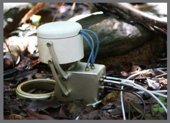
The eosMX-P multiplexer and eosAC autochambers can be interfaced with Los Gatos Research greenhouse gas analysers to create a fully automated soil flux measurement system with up to 12 chambers. The eosAC chambers open and close at user-defined intervals, and can be equipped with auxiliary sensors for soil moisture and temperature. Like the eosFD, the eosAC autochambers require very little power to operate, and are suitable for use in a variety of environments.
