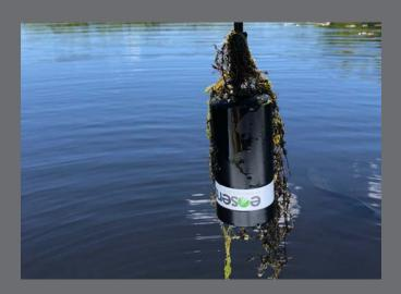
The eosGP waterproof CO<sub>2</sub> sensor packs the patented forced diffusion technology into a lightweight, portable sensor suitable for use in the field. The eosGP is submersible to a depth of 3 metres, allowing fluxes to be measured at various depths in a lake or river. Data can be logged via analog or RS-232, making the eosGP easy to integrate with other equipment. Eosense's software can even be used to log serial data on a laptop with the use of a USB serial converter.
