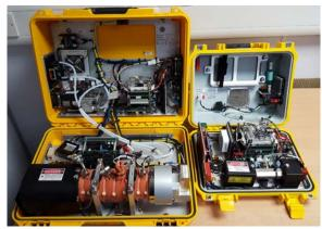
LGR have also released a few variations on the UGGA, which allow a fourth gas to be measured in addition to CH<sub>4</sub>, CO<sub>2</sub>, and H<sub>2</sub>O. Where the UGGA measures CH<sub>4</sub> & H<sub>2</sub>O on laser 1, and CO<sub>2</sub> on laser 2, these instruments measure CO<sub>2</sub> at a different absorption peak that is within the scanning range of laser 1, freeing up laser 2 for dedicated, precise measurements of a fourth gas.
